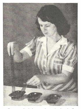
Emergency developing trays for small strips of roll film may be used as shown above. These are glass or Bakelite soap dishes available in five and dime stores.
