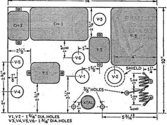
Panel and chassis layouts. The dimensions given should be followed carefully if the various parts indicated on the opposite page are used.
