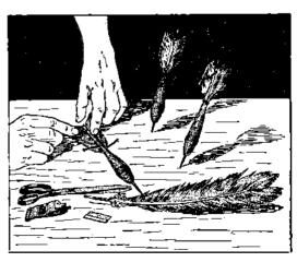
Point dart heads with finishing nails filed to needle points, then tack narrow bands of sheet lead around body for weight. Tails are then feathered with four 3-in. sections of feathers held in place with glue.
