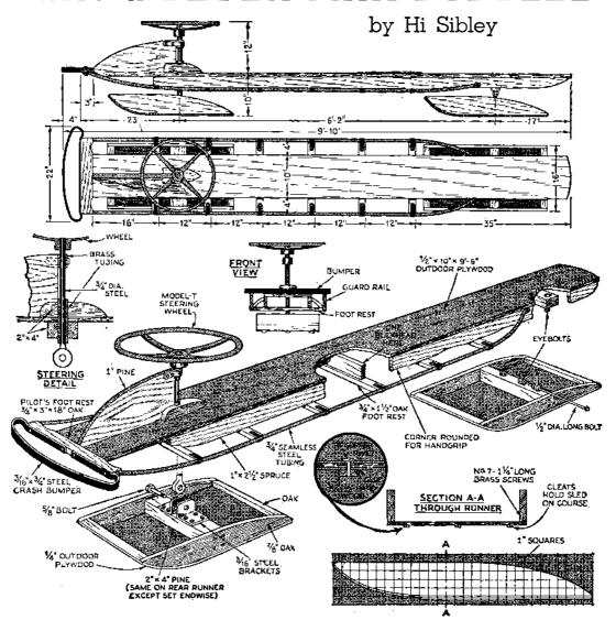
THIS novel bobsled, designed for virgin snow as well as the hard-packed runs, is exceptionally light without sacrifice of strength due to the use of outdoor plywood (Super-Harbord) for the plank and sleds. Two spruce side-members under the half-inch plywood plank form a box section of exceptional rigidity for the weight, and a seam-less-steel guard rail together with a crash bumper reduce the hazards of the slide.
