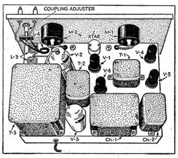
Back view of the "Compact Five" transmitter. Practically all the wiring is on the underside of the chassis.
