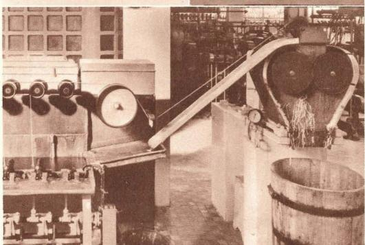
Casein in liquid form is forced through a platinum spmneret containing 600 minute holes. It then passes through a precipitating bath that solidifies it into filaments.
