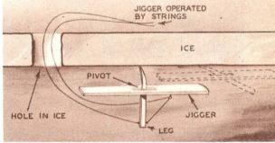
The "jigger" shown above illustrates how nets are placed under water. Pulling the strings causes the jigger to "walk" under the ice. When it has gone far enough it is located by its tapping noise, and a hole is dug and the jigger is removed. The cord attached to it is a continuous line from hole to hole, along which a net can be pulled under the ice.
