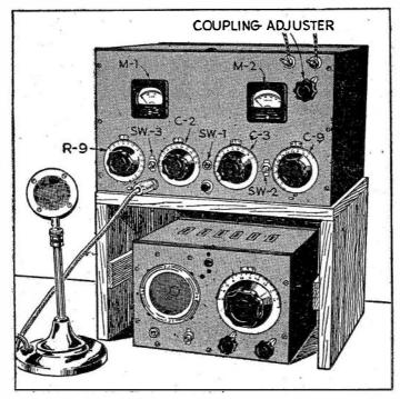
The "Compact Five" transmitter is the top unit, with the various controls marked to correspond with the schematic diagram on page 96. The pilot light under the switch SW1 lights when the high voltage switch SW3 is turned on. The bot-
