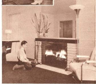
The efficiency of the living room fireplace is multiplied at least four times by a polished aluminum reflector placed behind the grate.
