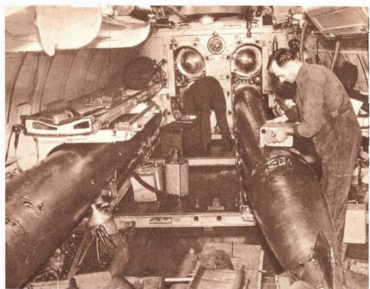
Interior of a torpedo room. Torpedoes are fired by the captain from the control room. He releases a charge of compressed air into the tube, ejecting the torpedo. As it slides out, a catch trips a trigger on the torpedo, starting the turbine and propellers.
