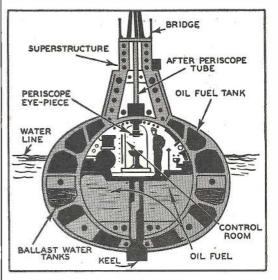
This is a cross section view of a British submarine, the X-1, which is 363 feet long, displaces 2,780 tons, and carries a crew of 109 men. Germany's "minnows" are one-third as long, have one-eleventh its displacement, and carry but onequartet of its crew.
