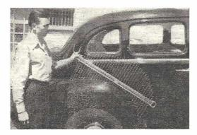
For measuring difficult contours on autos, planes or boats a tool with 34 feelers has been devised. When placed on any curved surface the feelers automatically fall into place and are kept in an accurate outline by locking the handle.
