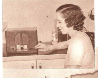
Above: This is "central" of the house communications system. Resembling a small radio receiver, the amplifier rests on a kitchen surface. From here one may speak to almost any other part of the house. Right: Another convenience is the electric blanket with its control box located on a convenient stand. Above the control box is a speaker-microphone unit of the communications system.
