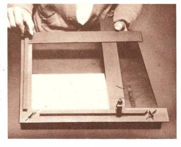
and the other at 45 degrees, as shown. Fasten wooden cleats on back of the base board, which should be about 17½ in. square and painted black. Cleats should be 34-in. stock 11/4-in. wide. Drill two holes at each end of the piano hinge and solder 118nuts to the underside. The exact point is determined by the location of the slots in the square. A thumb screw made from a 1/8-in. bolt, by soldering a part of a washer in the slot in the head, permits the square to slide freely.
