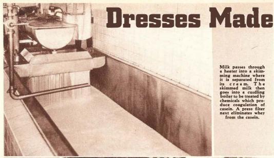
Milk passes through a heater into a skimming machine where it is separated from its cream. The skimmed milk then goes into a cutdling boiler to be treated by chemicals which produce cognitation of duce coagulation casein. A press filter next eliminates whey from the casein.
