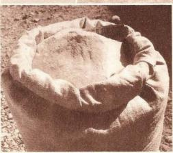
Casein appears in the form shown in the photo at left before it undergoes a dissolving process with chemical
